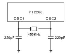
Unless any of the 8 keys (I1  $\sim$  I8) is being operated, the oscillation is automatically stopped. Thus, power consumption is considerably reduced.
