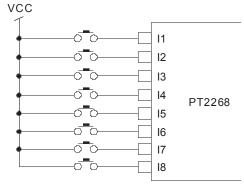
Furthermore, PT2268 has a built-in pull-low resistor of about  $60K \sim 110K\Omega$  which reduces the need for external components.
