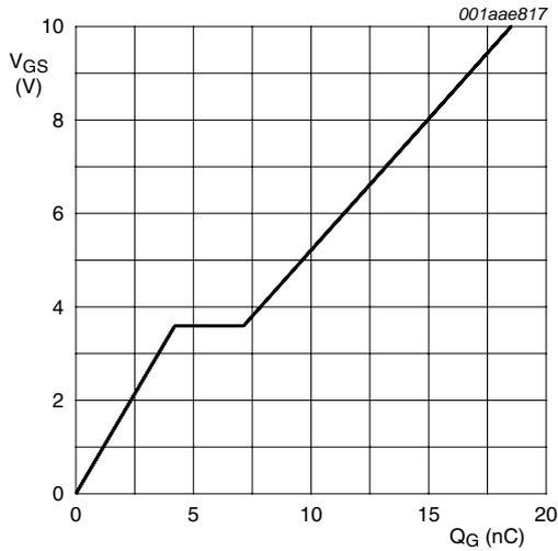
$I_D = 36\text{ A}; V_{DS} = 15\text{ V}$
