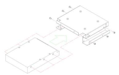
4. Secure the CD-ROM on the 3-in-1 drive bay after fastening it onto a transfer card.
