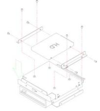
6. The fully-equipped, 3-in-1 drive bay is placed on the BPC-6670 by means of screw.
