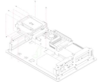
2. Remove the 3-in-1 drive bay in accordance with the picture.
