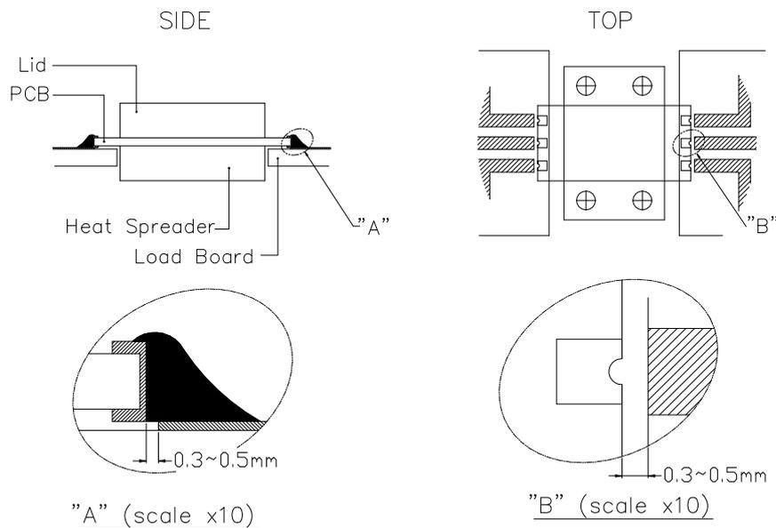
★ It can be easily removed with solder wick and other removable material.
