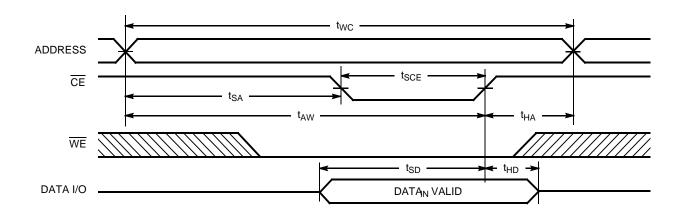
Write Cycle No. 3 ( $\overline{\text{WE}}$  Controlled,  $\overline{\text{OE}}$  LOW)<sup>[5, 9, 14]</sup>
