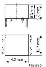
Recommended hole arrangement (view in mounting direction)
