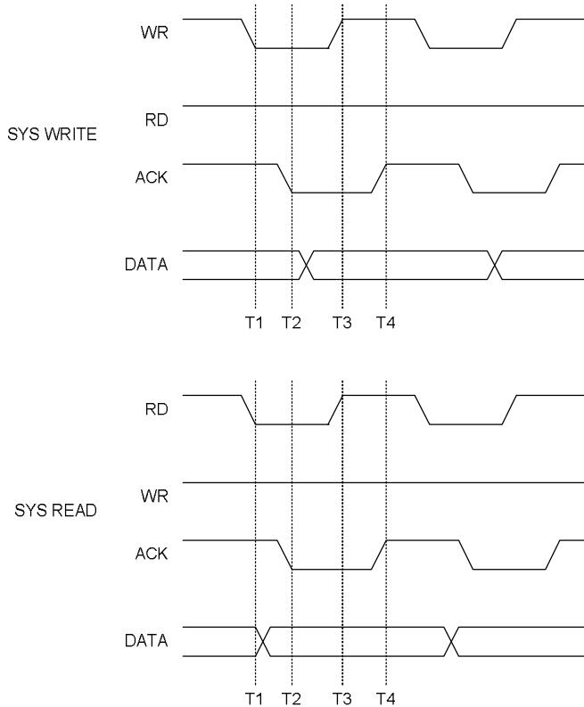
Note: WR (pin 31), RD (pin 32) is controlled by system (master controller), and ACK (pin 28) is controlled by SC9641 (sub-controller), normal state is high level, and DATA is controlled by all above.
