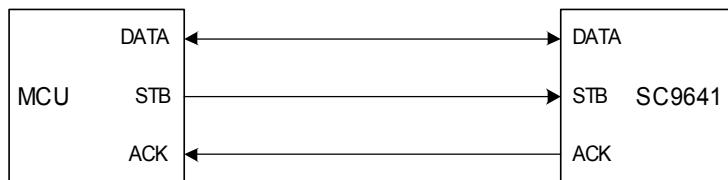
DATA (pin 31): synchronization and data transmission.
