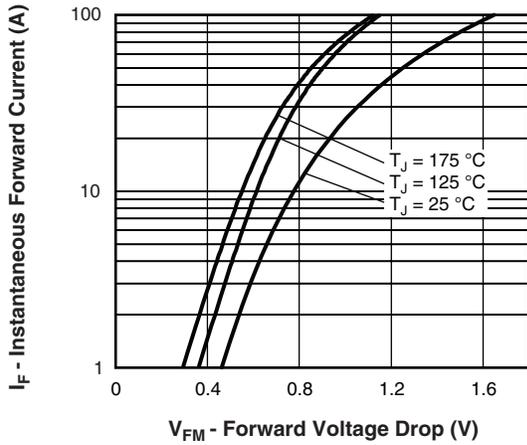
Fig. 1 - Maximum Forward Voltage Drop Characteristics
