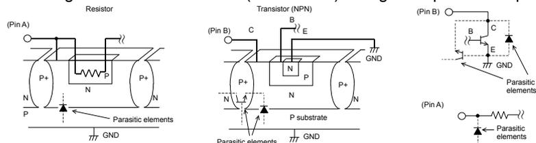
Fig.9 Example of a Simple Monolithic IC Architecture
