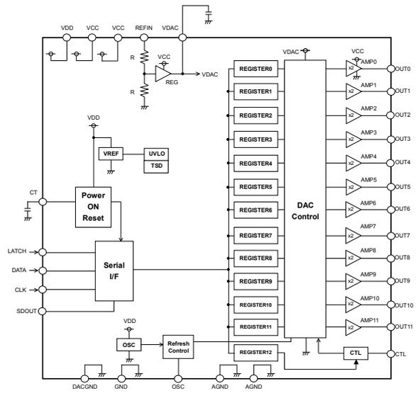
Fig.1 Pin No. & Block Diagram
