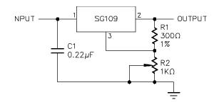
FIGURE 2 - ADJUSTABLE OUTPUT REGULATOR
