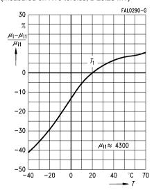
Initial permeability  $\mu_i$ versus temperature (measured on R10 toroids,  $\hat{B} \leq 0.25$  mT)
