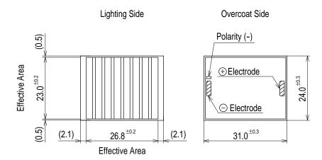
Note: Glass Substrate Thickness : 1.1mm Module Thickness : 1.3mm max Accepts normal soldering for bending.
