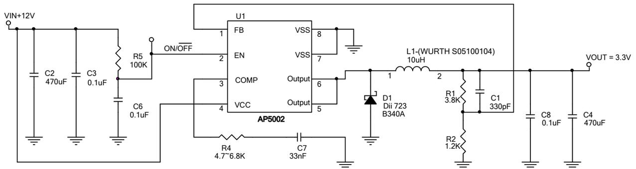
Notes: 4.  $V_{OUT} = V_{FB} \times (1 + \frac{R1}{R2})$
