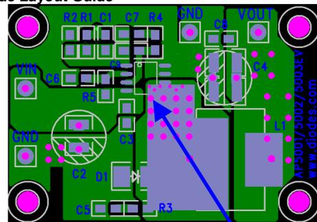
Use vias to conduct the heat into the backside of PCB layer. The PCB heat sink copper area should be solder-painted without masked. This approaches a
