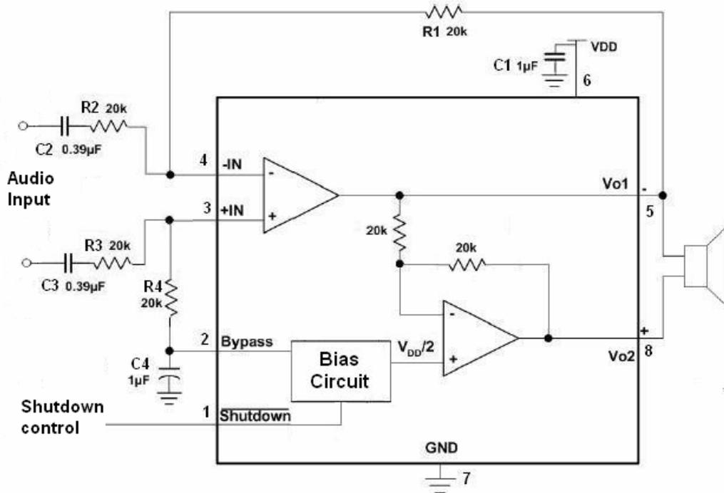
**Figure 2. Audio Amplifier with Differential Input**
