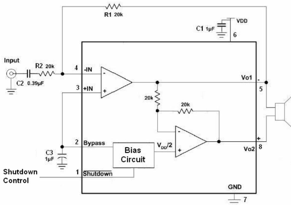
**Figure 1. Audio Amplifier with Single –Ended Input**
