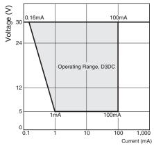
However, even when using microload models within the operating range shown above, if inrush current or inductive voltage spikes occur when the contact is opened or closed, then contact wear may increase and so decrease the service life. Therefore, insert a contact protection circuit where necessary.
