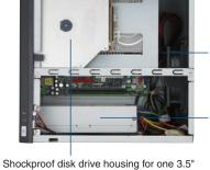
HDD and one slim-type optical drive
