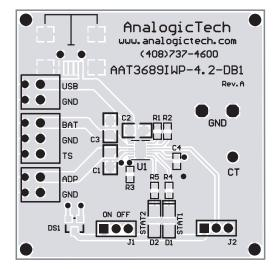
Figure 5: AAT3689 Evaluation Board Component Side Layout.
