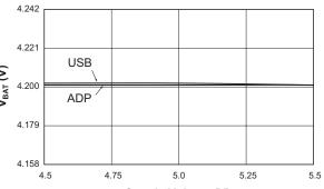
Battery Voltage vs. Supply Voltage
