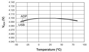
**Preconditioning Voltage Threshold** vs. Temperature
