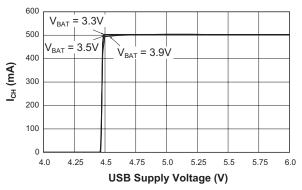
Fast Charge Current vs. Adapter Supply Voltage  $(R_{SETADP} = 8.06k\Omega)$
