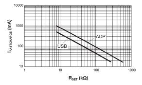
Figure 2: I<sub>FASTCHARGE</sub> vs. R<sub>SET</sub>.
