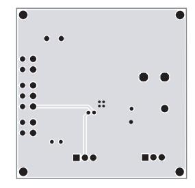
Figure 6: AAT3689 Evaluation Board Solder Side Layout.
