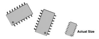
Vishay Thin Film offers standard circuits in 16 pin in a medium body molded surface mount package. The networks are available over a resistance range of 100 ohms to 100K ohms. The network features tight ratio tolerances and close TCR tracking. In addition to the standards shown, custom circuits are available upon request.
