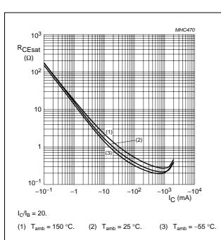
Fig.8 Collector-emitter equivalent on-resistance as a function of collector current; typical values.
