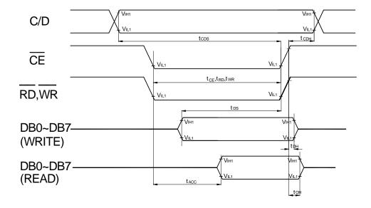
Fig. a Interface timing (data write/read)
