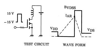
$$\begin{aligned} R_G &= 25~\Omega \\ V_{DD} &= 90~V,~L = 7.5~mH \end{aligned} \qquad E_{AS} &= \frac{1}{2} \cdot L \cdot I^2 \cdot \left( \frac{B_{VDSS}}{B_{VDSS} - V_{DD}} \right) \end{aligned}$$
