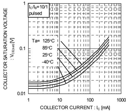
Fig.6 Collector-Emitter Saturation Voltage vs Collector Current ( II )
