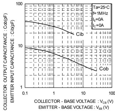
Fig.10 Emitter input capacitance vs. Emitter-Base Voltage
