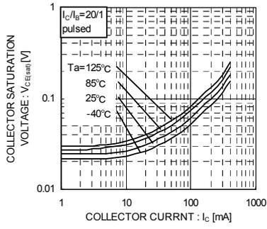
Fig.7 Collector-Emitter Saturation Voltage vs Collector Current (III)
