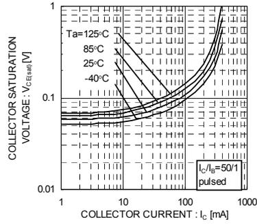
Fig.8 Collector-Emitter Saturation Voltage vs Collector Current (IV)
