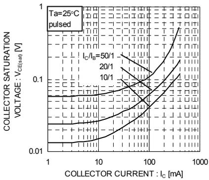
Fig.5 Collector-Emitter Saturation Voltage vs Collector Current ( I )
