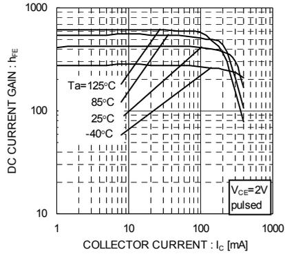
Fig.4 DC Current Gain vs Collector Current ( II )
