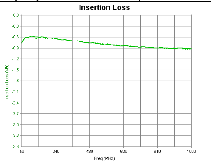
Figure 4 The Balun with an external 100 pF capacitor to enhance insertion and return loss. Data is compared to the basic Guanella configuration (dashed lines). Other capacitor values can be used with different results.
