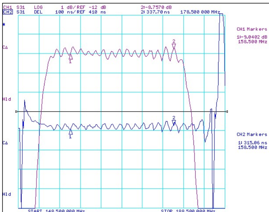
Fig. 2 Horizontal : 4MHz/Div Vertical: 1dB/Div Vertical: 100nS/Div
