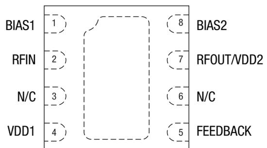
**Figure 2. SKY65049-360LF Pinout – 8-Pin QFN (Top View)**
