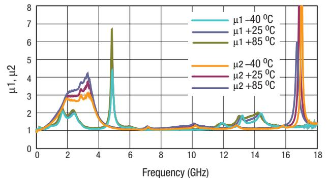
Figure 10. Stability vs Frequency Over Temperature ( $P_{IN} = -20$  dBm)
