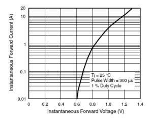
Figure 3. Typical Forward Characteristics Per Diode
