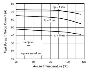
Figure 6. Non-Repetitive Peak Forward Surge Current Square Waveform
