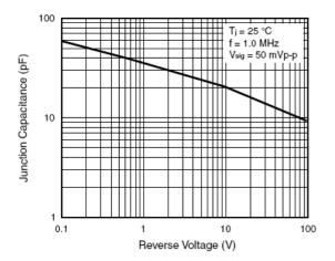
Figure 5. Typical Junction Capacitance Per Diode
