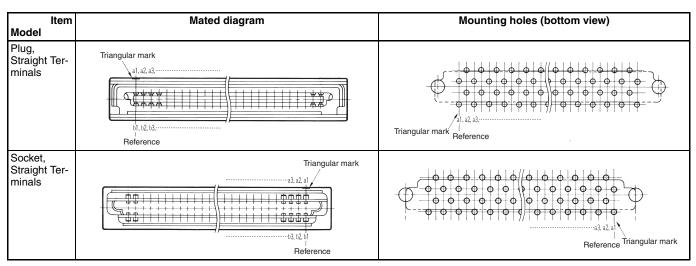
Note: 1. Contact numbers are not printed on the connectors. Use the triangular mark (▼) as a guide when designing and mounting to boards.
