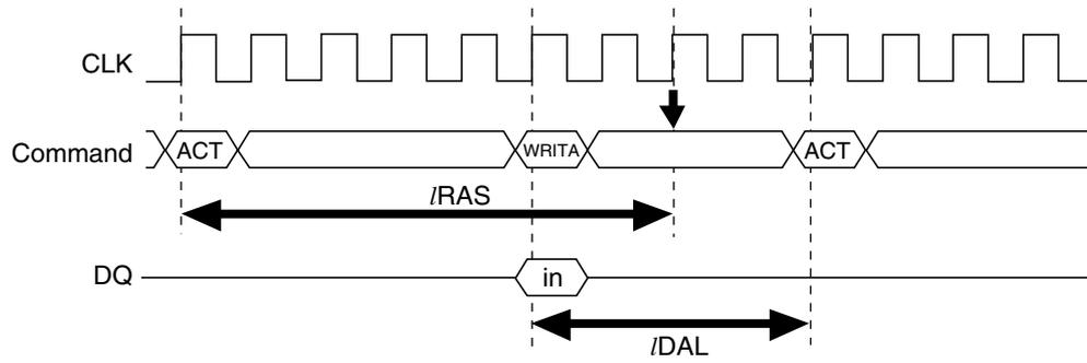
Note: Internal auto-precharge starts at the timing indicated by "↓", and an interval of  $t_{RAS}$  ( $/RAS$ ) is required between previous active (ACT) command and internal precharge "↓".
