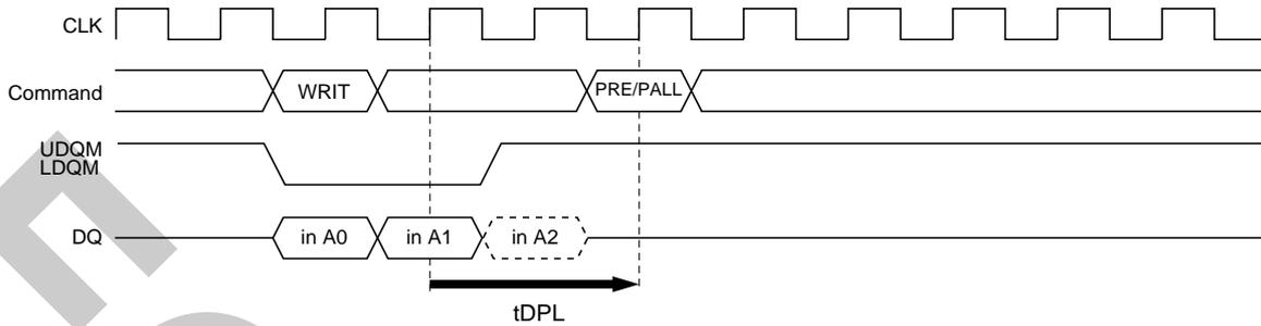
**WRITE to PRECHARGE Command Interval (same bank) (BL = 4 (To stop write operation))**
