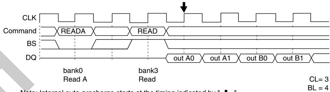
**Read with Auto Precharge to Read Command Interval (Different bank)**
