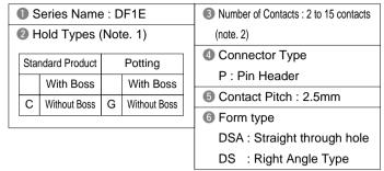
Note 1: The right angle pin header has no symbol. Note 2: The potting header has 2 to 10 contacts.
