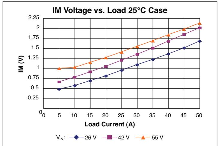
Figure 8 – IM voltage vs. load; 25°C Case
