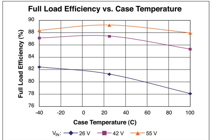
Figure 2 – Full load efficiency vs. temperature;  $V_{IN}$
