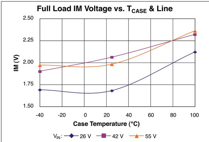
Figure 9 – Full load IM voltage vs.  $T_{CASE}$  & line
