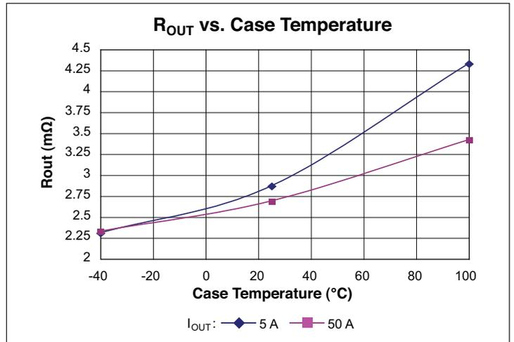
Figure 4 –  $R_{OUT}$  vs. temperature vs.  $I_{OUT}$
