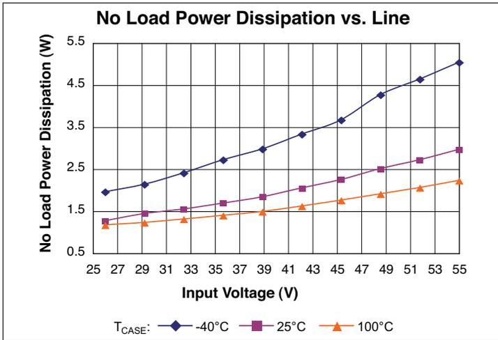
Figure 1 – No load power dissipation vs.  $V_{IN}$ ;  $T_{CASE}$
