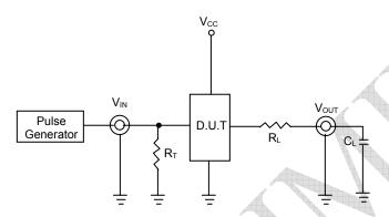
C<sub>L</sub> = 15pF Test Circuit
