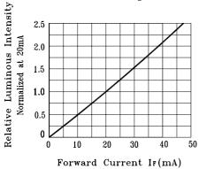
Fig.4 Relative Luminous Intensity vs. Forward Current
