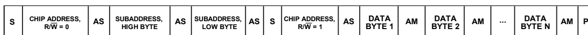
S = START BIT, P = STOP BIT, AM = ACKNOWLEDGE BY MASTER, AS = ACKNOWLEDGE BY SLAVE. SHOWS A ONE-WORD READ, WHERE EACH WORD HAS N BYTES.
