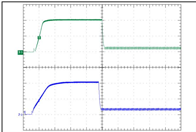
**Figure 19:** Load current (10A/div) as a function of time (500uS/div) when attempting to turn on into a 10 mΩ short circuit. \*-Output voltage setpoint is trimmed to 5.25V for the top trace and 0.7V for the bottom trace.
