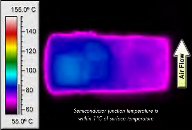
**Figure 7:** Thermal plot of 2.5Vo converter at 12.0Vin with 7 amp load current and 55°C. Air is flowing across the converter from pin 1 to 11 at 200 LFM.
