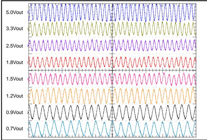
**Figure 13:** Output Voltage Ripple at 12V input voltage and rated load current (10 mV/div). Load capacitance: 5 ceramic 22 $\mu$ F capacitors. Bandwidth: 20 MHz. See Figure 17.
