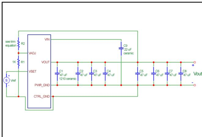
**Figure 17:** External cap shown for transient response measurements. Not shown are PWRGOOD output and digital inputs OE, TRIMN and TRIMP. I/O pin arrangement not intended to match positions on the converter.
