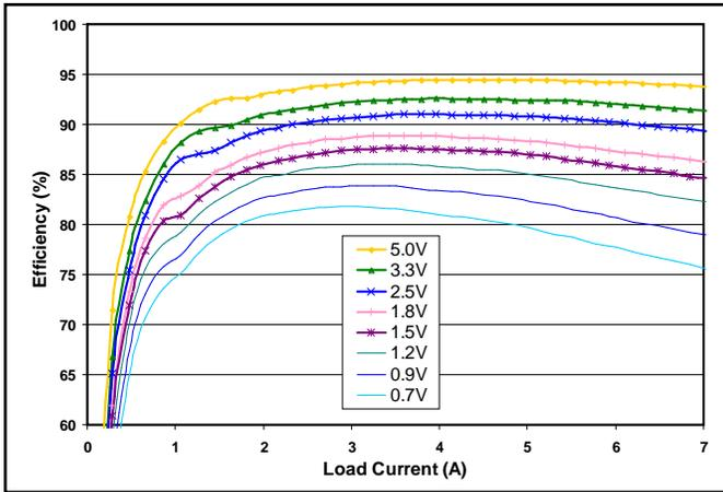
**Figure 1:** Efficiency at 12Vin and nominal output voltage vs. load current for CCM modules at 25°C (see [Continuous vs Discontinuous Conduction](#) app note).
