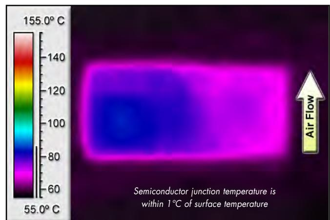
**Figure 6:** Thermal plot of 0.9Vo converter at 12.0Vin with 7 amp load current and 55°C. Air is flowing across the converter from pin 1 to 11 at 200 LFM.
