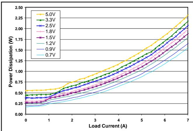
**Figure 3:** Power dissipation at 12Vin and nominal output voltage vs. load current for CCM modules at 25°C (see [Continuous vs Discontinuous Conduction](#) app note).
