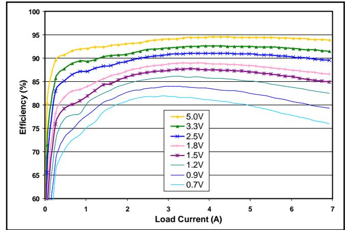
**Figure 2:** Efficiency at 12Vin and nominal output voltage vs. load current for DCM modules at 25°C (see [Continuous vs Discontinuous Conduction](#) app note).
