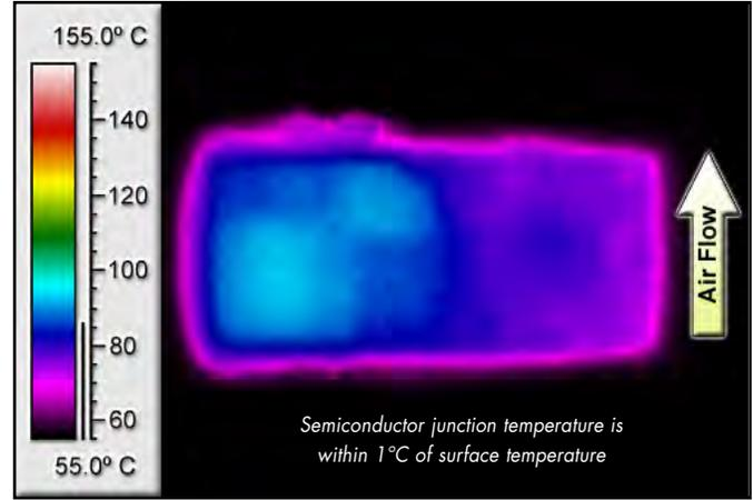
**Figure 8:** Thermal plot of 5.0Vo converter at 12.0Vin with 7 amp load current and 55°C. Air is flowing across the converter from pin 1 to 11 at 200 LFM.
