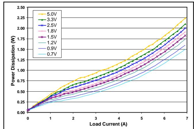
**Figure 4:** Power dissipation at 12Vin and nominal output voltage vs. load current for DCM modules at 25°C (see [Continuous vs Discontinuous Conduction](#) app note).
