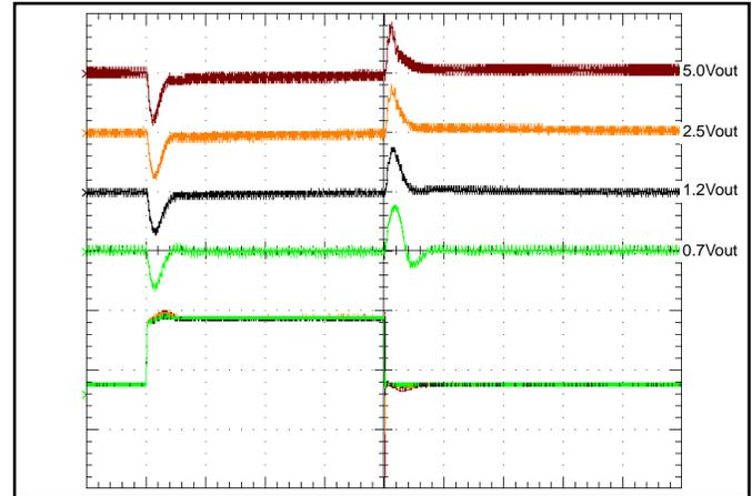
**Figure 10:** CCM (QS3 & QS4) output voltage response at 12.0Vin to step-change in load current (10% to 90% of Iout max; di/dt=20A/μs; 50μs/div). Load cap: 376μF ceramic. Top: Vout (100mV/div), Bottom: Iout (5A/div).
