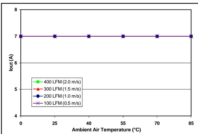
**Figure 5:** Maximum output power derating curves vs. ambient air temp for all output voltages at 12Vin. Airflow rates of 100 - 400 LFM with air flowing across the converter from pin 1 to 11..
