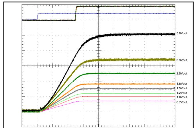
**Figure 12:** CCM (QS3 & QS4) turn-on transient at 12Vin and full load (resistive load) with 370uF of output cap (1V/div, 1mS/div), top traces are OE pin (first to rise) and PWRGOOD (rising later), both at 5V div.
