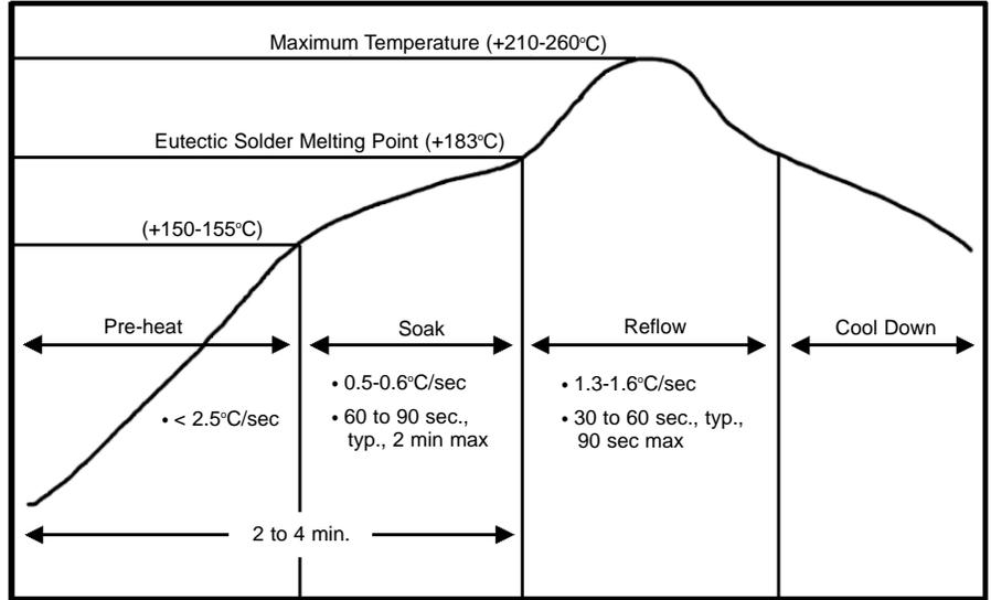
Figure J: Typical Eutectic (96.5Sn/3.0Ag/0.5Cu) Solder Profile
