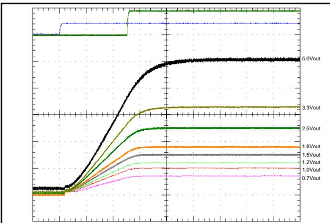
**Figure 11:** DCM (QS1 & QS2) turn-on transient at 12Vin and full load (resistive load) with 370uF of output cap (1V/div, 1mS/div), top traces are OE pin (first to rise) and PWRGOOD (rising later), both at 5V div.
