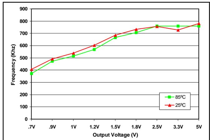
**Figure 18:** Typical Switching Frequency vs Output Voltage, 12Vin, Full Rated Load Current.
