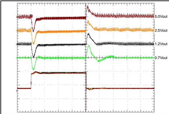
**Figure 9:** DCM (QS1 & QS2) output voltage response at 12.0Vin to step-change in load current (10% to 90% of Iout max; di/dt=20A/μs; 50μs/div). Load cap: 376μF ceramic. Top: Vout (100mV/div), Bottom: Iout (5A/div).
