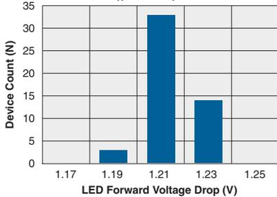
**Typical On-State Output Voltage Drop Distribution**
