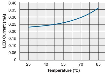
**Typical Leakage vs. Temperature**
