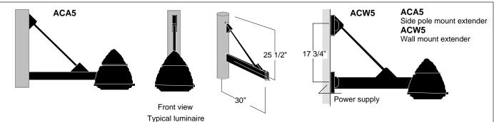
ACA5 -EPA: 0.8 1" X 3" extruded aluminum side pole arm mount. 4" O.D X 30" lg. post top adaptor with a cast aluminum tenon to fit with a 3 3/4" I.D. pole. 1/2" dia. stainless steel rod support. Extruded arm and all other parts are painted same color as Luminaire.
