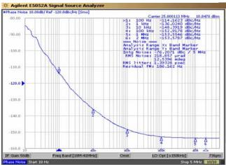
Phase noise of the reference signal, Out3. 25MHz Reference Frequency
