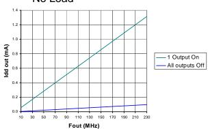
FD5 Series I<sub>DD</sub> versus PLLs Used  $V_{DD}=1.8V$
