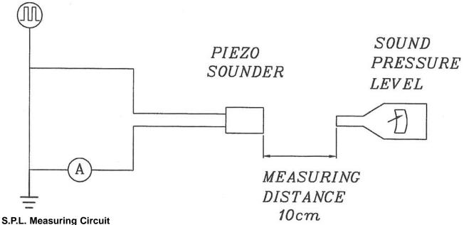
Input Signal: 10 Vp-p, 4.0 KHz, Square Wave
