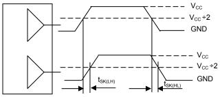
The pin-to-pin skew is defined as the worst case difference in propagation between any similar delay path within a single device
