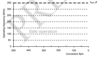
Figure 15. No maximum frequency limitation for V<sub>cc</sub> = 3.3V, MTBF 4 years, driving series terminated transmission lines, 2s2p board
