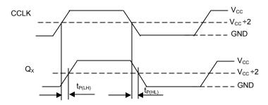
Figure 6. Propagation Delay (t<sub>PD</sub>) Test Reference
