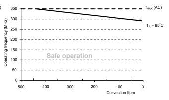
Figure 16. Maximum PCS2I99447 frequency V<sub>CC</sub> = 3.3V, MRBF 4 years, 4pF load per line, 2s2p board
