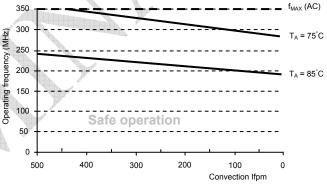
Figure 14. Maximum PCS2I99447 frequency V<sub>CC</sub> = 3.3V, MRBF 9.1 years, 4pF load per line, 2s2p board
