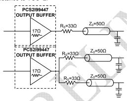
Figure 2. Single versus Dual Transmission Lines
