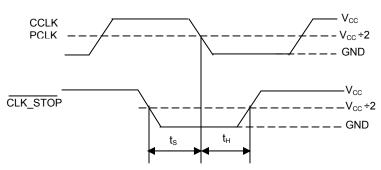
Figure 12. Setup and Hold Time (t<sub>s</sub>, t<sub>h</sub>) Test Reference
