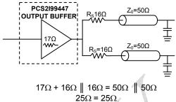
Figure 4. Optimized Dual Line Termination
