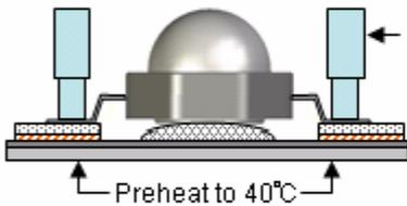
**Hot bar soldering of LED emitter**
