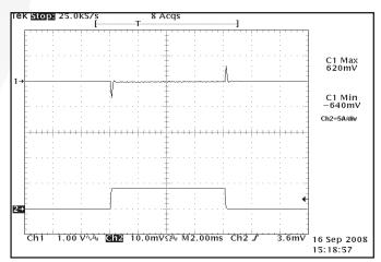
**Figure 12:** Output voltage response to step-change in load current 0%-50%-0% of Iout (max). Load cap:  $1\mu$ F ceramic cap and  $10\mu$ F, 100 m $\Omega$  ESR tantalum cap. Ch 1: Vout (1V/div). Ch 2: Iout (5A/div).
