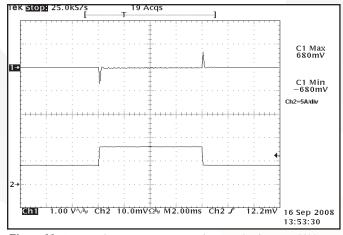
**Figure 11:** Output voltage response to step-change in load current 50%-100%-50% of Iout (max). Load cap:  $1\mu$ F ceramic cap and  $10\mu$ F, 100 m $\Omega$  ESR tantalum cap. Ch 1: Vout (1V/div). Ch 2: Iout (5A/div).
