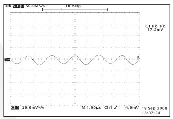
**Figure 16:** Output voltage ripple, Vout, at nominal input voltage and rated load current (20 mV/div). Load capacitance:  $1\mu$ F ceramic capacitor and  $10\mu$ F tantalum capacitor. Bandwidth: 10 MHz. See Figure 14.
