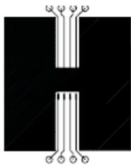
a) 78°C/W when mounted on a 0.5 in<sup>2</sup> pad of 2 oz copper
