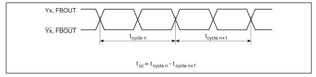
Figure 5 Cycle to cycle jitter
