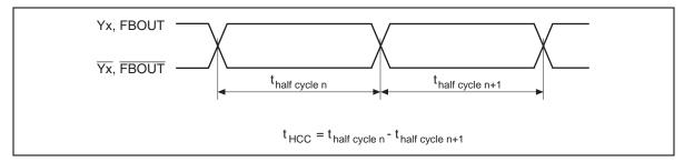
Figure 8 Half cycle to cycle jitter
