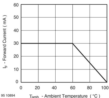
Figure 2. Forward Current vs. Ambient Temperature for InGaN
