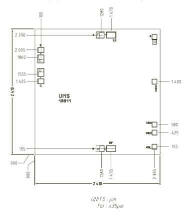
**Bonding pad positions** (Chip thickness: 100µm. All dimensions are in micrometers)
