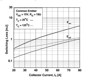
Figure 14. Turn-on Characteristics vs. Collector Current
