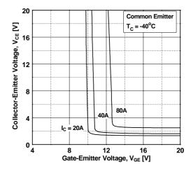
Figure 7. Saturation Voltage vs. V<sub>GE</sub>
