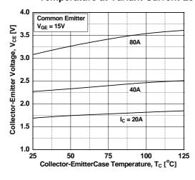
**Figure 2. Typical Output Characteristics**
