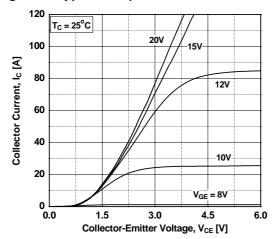
Figure 3. Typical Saturation Voltage Characteristics
