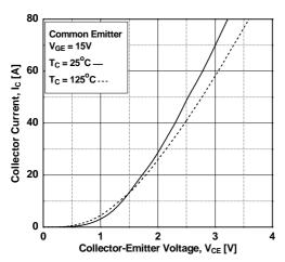
Figure 5. Saturation Voltage vs. Case
