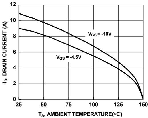
Figure 11. Maximum Continuous Drain Current vs Ambient Temperature
