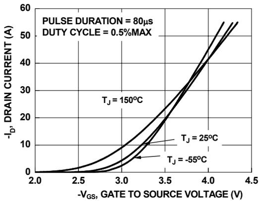
Figure 5. Transfer Characteristics
