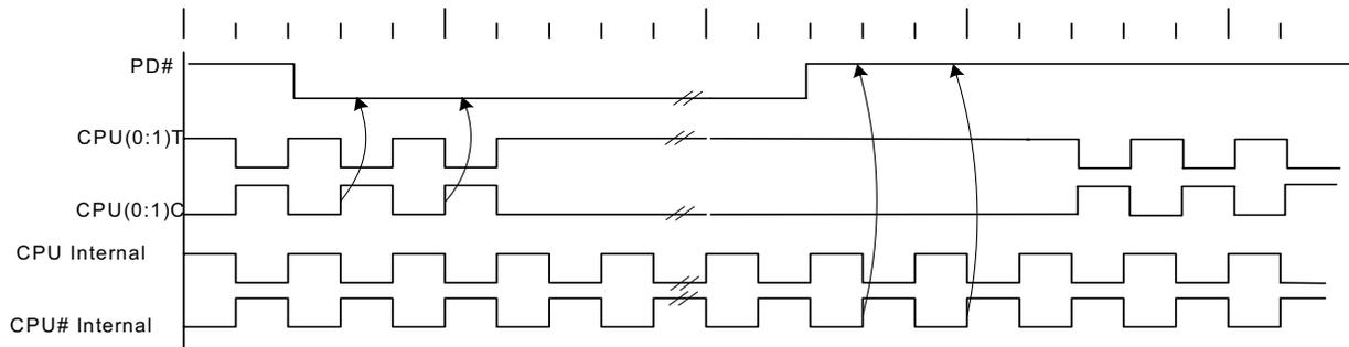
**Figure 5. Power-down Assertion/Deassertion Timing Waveforms – Nonbuffered Mode**
