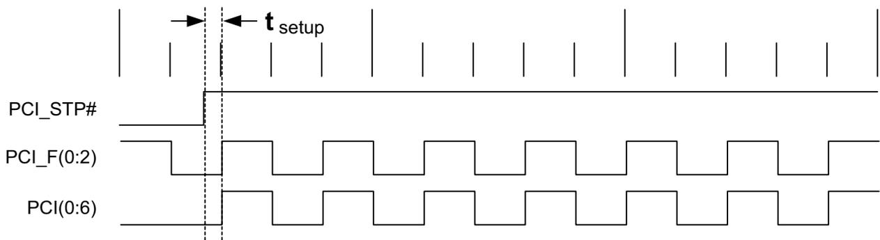
**Figure 4. Deassertion PCI\_STP# Waveform<sup>[7]</sup>**
