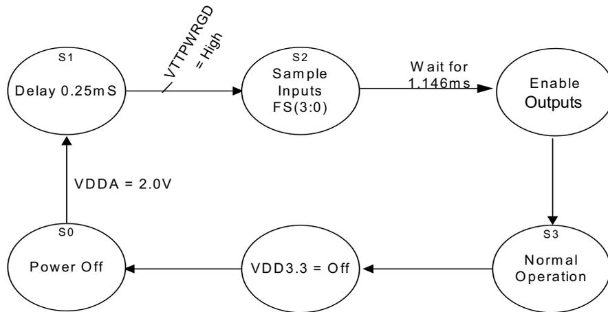
Figure 7. Clock Generator Power-up/Run State Diagram
