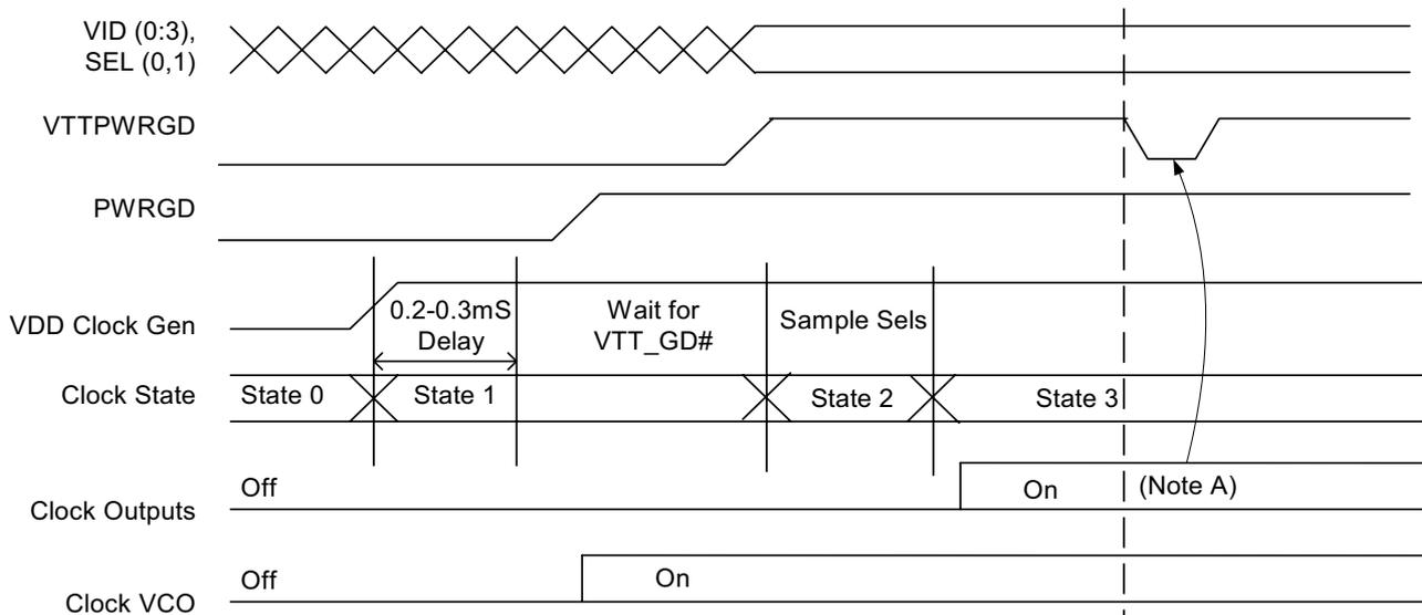
**Figure 6. VTT\_PWRGD Timing Diagram<sup>[8]</sup>**
