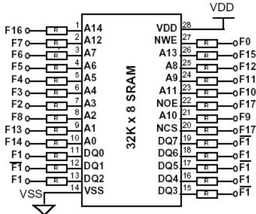
VDD = 5.6V,  $R \leq 10\text{ K}\Omega$ ,  $V_{IH} = V_{DD}$ ,  $V_{IL} = V_{SS}$
