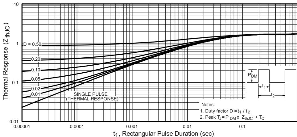
Fig. 4 - Maximum Thermal Impedance  $Z_{thJC}$  Characteristics (Per Leg)
