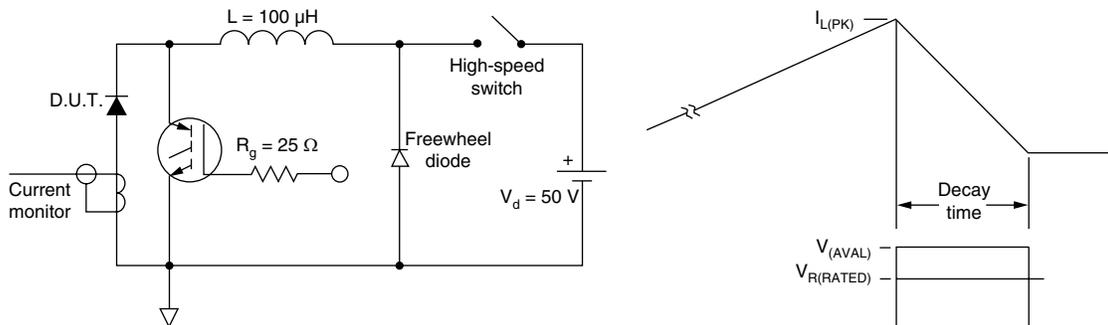
Fig. 11 - Avalanche Test Circuit and Waveforms
